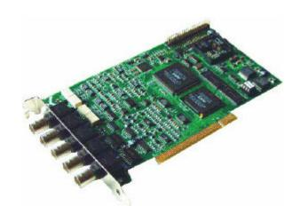
The Acquitek C H3160 Series of High Speed Data Acquisition Boards was designed to provide superior high-speed functionality and performance at a low price. All CH Series boards utilize 16 MB of onboard memory, a local processor, and PCI bus mastering to provide glitch-free capture and/or playback of analog signals of length limited only by host RAM size, even with a non-realtime PC operating system.
